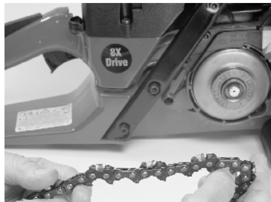
Fig. 25. Inspect the chain
