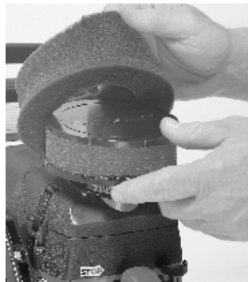
Fig. 33. Remove the Pre-filter
