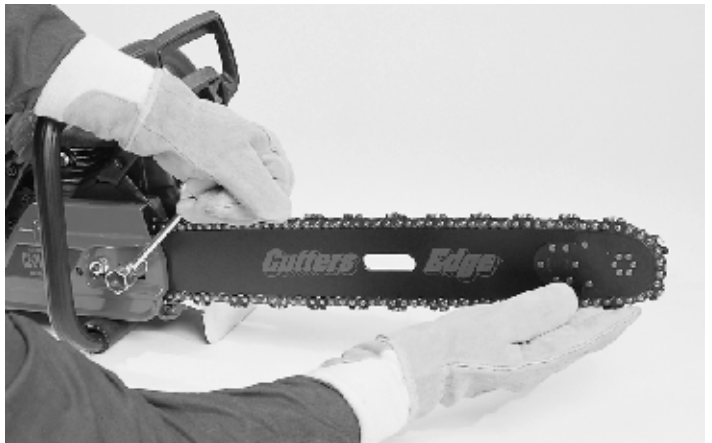
Fig. 8. Tighten two clutch cover nuts so chain is at proper tension
