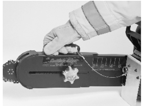
Fig. 21. Set to the desired depth of cut.
