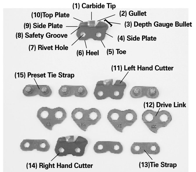
Fig. 26. Components of the BULLET® CHAIN
